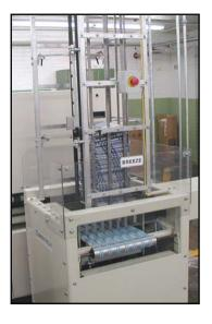
The Breeze II accurately folds pillow shams of various material types and sizes. Folded shams are stacked by a high capacity stacker.
