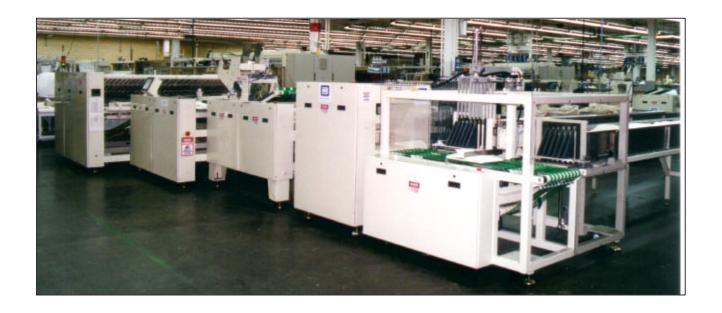
The Orion folds fitted sheets of various material types including poly/cotton, sateen and flannel. Sheet sewing pattern can be length for length or width for length. A cardboard can be inserted in the 2<sup>nd</sup> crossfold. Our *Pressing Unit* presses down folded items, enhancing package quality.
