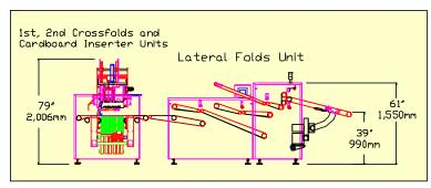
The Stealth folding system provides high quality folds of flat sheets including flannel, satin, sheets with ruffles/piping; showing or hiding the border. A cardboard can be inserted in the 1<sup>st</sup> crossfold. Folding capacity is up to 900 sheets/hour.
